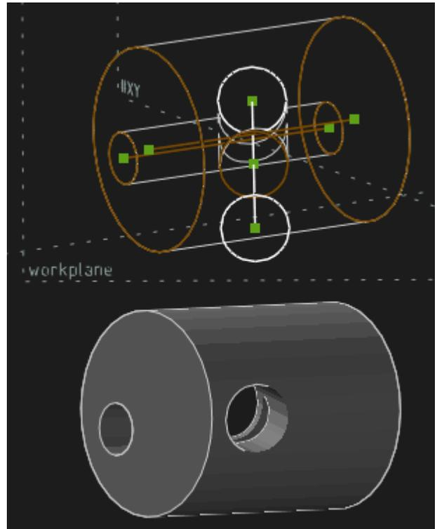
The image at right shows a difference-extrusion solid made with an oblique workplane. The 1st cylinder, with a longitudinal shaft through it, was extruded in Z from 2 concentric circles in XY. Then another cylinder was extruded from another circle in a new, oblique workplane to punch a new, slanted shaft through the first cylinder and intersect its shaft.
