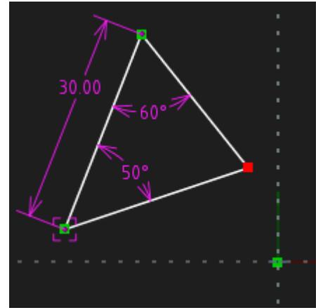
If an error does arise, the "simplest restriction" approach should yield an answer. If not, then you finally have to try to find a different constraint (or mix of constraints) that restricts fewer DOFs. Most constraints restrict 1 DOF, some restrict 2, and some in 3D restrict 3.
