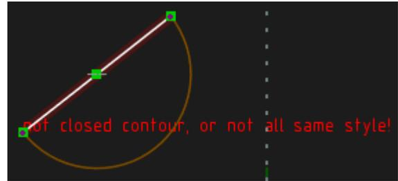
Joining a line in a new group to a linked-in arc doesn't close the arc (nor the line).
