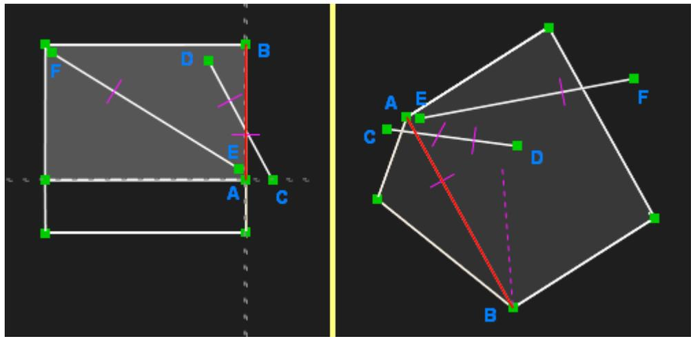
and a circle in a workplane, while in 3D mode. So, the point is only limited to the circle's projection in 3D (a cylinder--of infinite length). I extruded the circle, as shown in the rotated view on the right, just to help illustrate this. The point can move anywhere in free space, as long as it stays on the surface of that cylinder.
