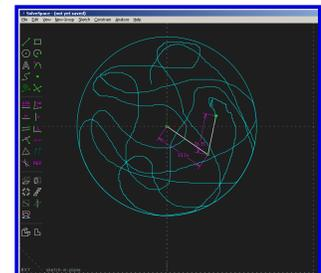
The particular usefulness of the SolveSpace linkage solver is that the parts of a 3D model (designed to move) can be checked for interference as the "skeleton" defined by their linkages is actuated through its range of motion, and have that motion recorded.
