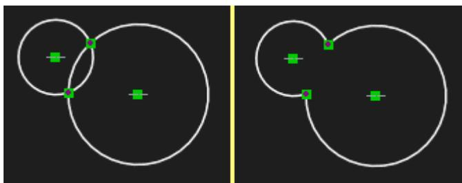
Like Tangent Arcs, any constraints the intersecting lines/curves had are lost. If you mark a participating line/curve as **construction** before the Split, then it gets "left behind" with any constraints, and the split gets applied to a copy of it, as non-construction geometry.
