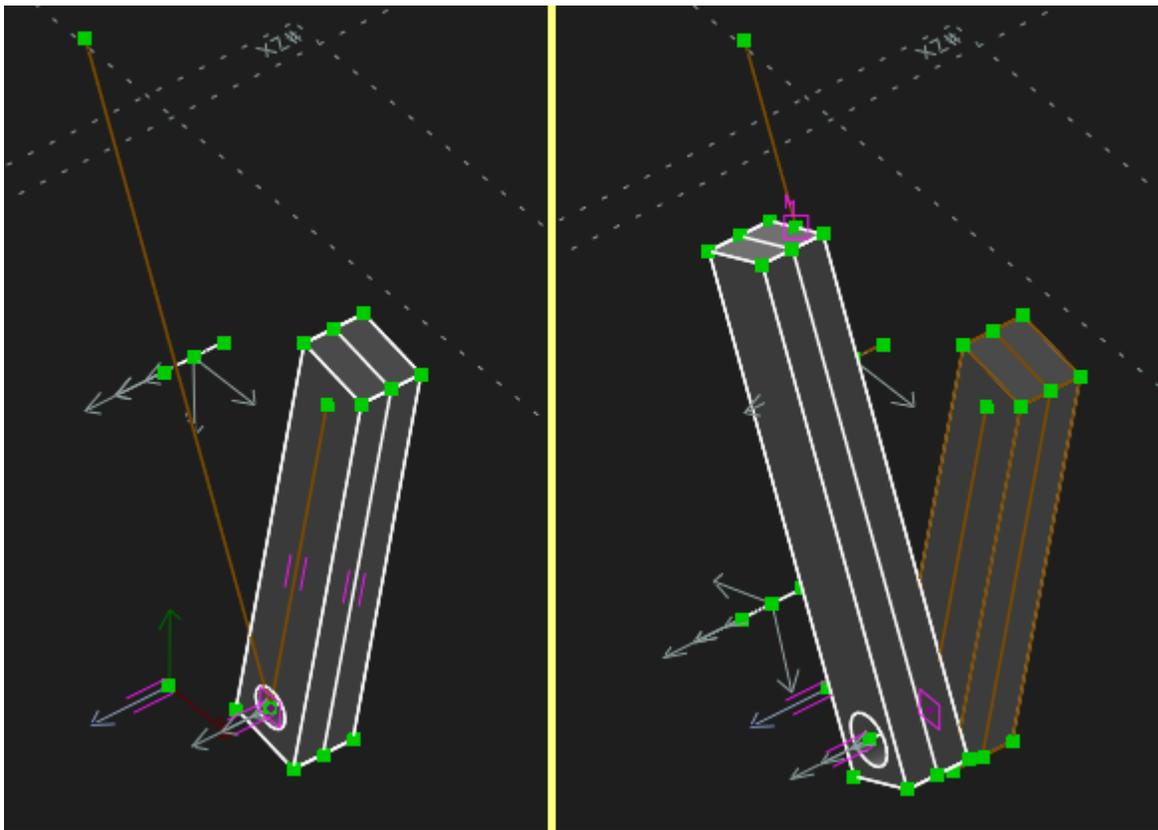
Next, shown on the right, a 2nd bar was linked in. The same first 3 constraints were created on it (but using the hole center on its back face in this image). To connect its movement with the other linkage line, a point-on-line constraint was made between a midpoint on its top-back edge and the line (indicated with a purple "M" and square). The linkage group could then be activated and moved to test both it and the model.
