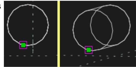
Note, also, that constraints function across workplanes (and groups). If the point in the last example above was in a workplane (different than the circle's), it would be constrained to move along the (elliptical) intersection of the circle's cylindrical projection with that workplane. Because both objects are limited to 2D, whether the constraint was made in 2D or 3D mode wouldn't matter.
