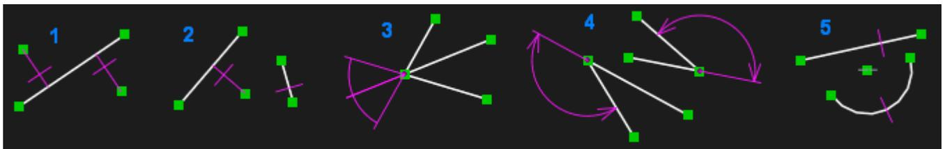
If points of a shape are dragged too quickly, the solver may change the shape of contour while checking constraints. Try dragging slower, or moving it in increments (or using **Analyze > Step Dimension** to increment it automatically).
