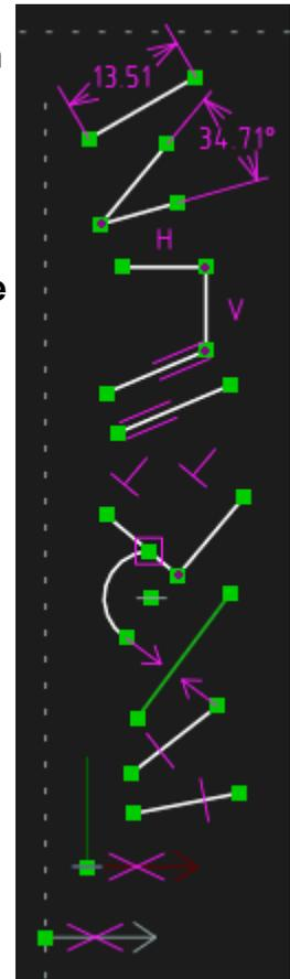
Constraints can be selected for taking action on them, for example to delete or change parameters.
