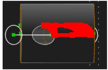
If the errors keep showing up every time you activate an extrusion group, you can set its **force NURBS surfaces to triangle mesh** option in **Property Browser** to prevent them. This tells the solver to use the finite-lines approximation (mesh) of the shape instead of its exact NURBS mathematical definition (and therefore be more forgiving).
