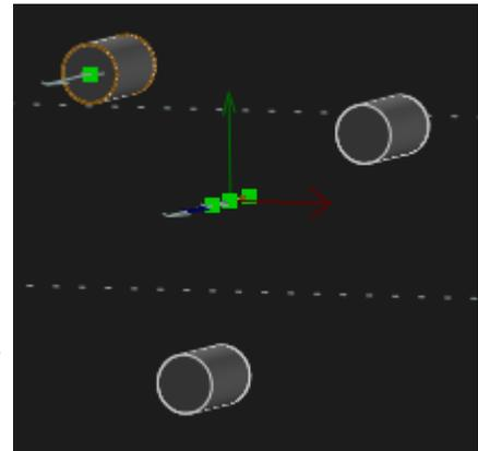
Notice that, with both translating and rotating, the spacing of the copies can be made exact with a constraint (distance or angle, respectively).
