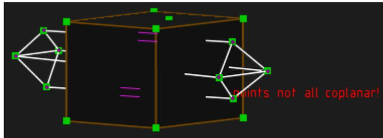
To construct complex 3D objects, it's best to create separate objects in separate workplanes, then extrude the objects to merge them (rather than drawing freehand in 3D). You can draw meshes with freehand 3D contours but it's not easy. And SolveSpace won't draw shaded surfaces for them, whether with coplanar points or not.
