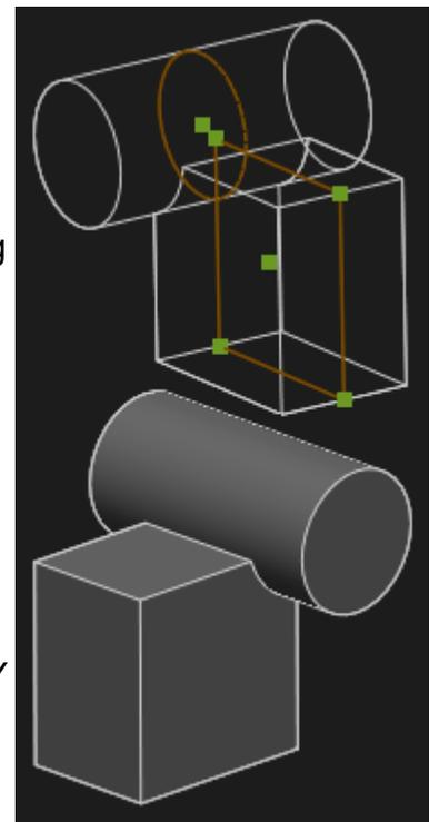
The path of extrusion is always normal to the active workplane. If you have a typical contour in XY, then make YZ active for example, and extrude (along X), you'll get a flat mess filled with errors.
